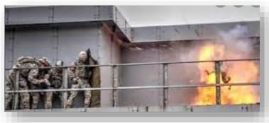
Blast Overpressure Reduction (BOR) Form used in breaching operations with det cord or malleable explosive to reduce Soldiers & Instructor blast overpressure exposure by 20%-50%
